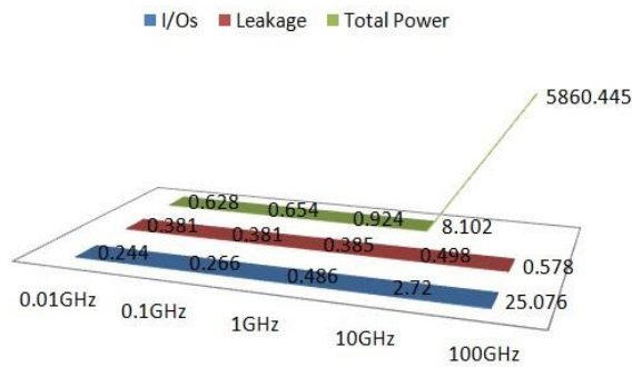
Fig. 5. Chart of I/Os, Leakage and Power at different frequencies for HSTL-III
