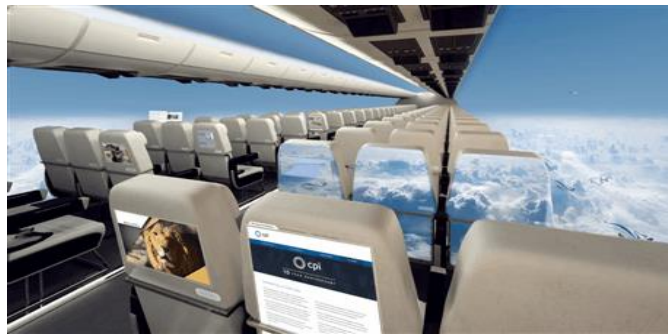
Fig.1: Thin lining of screens on fuselage as well as on back of seats [1]
